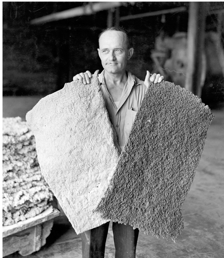
A worker at B. F. Goodrich showing that sheets of synthetic rubber (left) and natural rubber (right) are nearly identical except for their color
